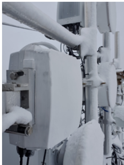
Antenna with water-repellent coated radome
