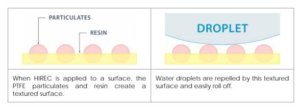
**HIREC 100** is a water-repelling material with anti-fouling properties. It is most effective in protecting against damage from water and snow, and its water-repelling performance last for approximately 3 years. NOTE: HIREC 100 requires the application of a primer coating
