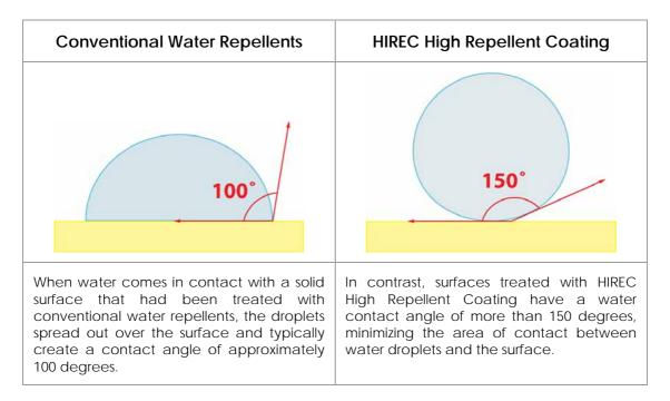
This is achieved as a result of the unique composition of the HIREC coating material, which combines miniscule PTFE particulates and a fluorinated resin. When applied to a solid surface, the particulates and resin disperse to create a textured surface; when this surface is exposed to water, the droplets come in contact only with the raised particulates and easily roll off.
