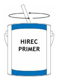
Note: When mixing whole cans of the HIREC Primer UP Base and Hardener, the proper mixing ratio will be achieved. If you are using only a portion of the Primer UP Base, use a weight scale to measure accurate amounts of each to achieve the proper mixing ratio, and immediately seal up the remaining materials. Mix according to weight ratio, not volume ratio.
